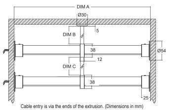
/CP - Coupler is required when the hanging rail exceeds 3m. In this case 2 lengths will be supplied and the coupler hides the join allowing up to a 6m hanging rail. Cable entry will be required at both ends. See page 3 for details. Specify Dim A and B
